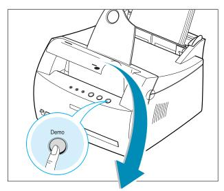
The demo page provides a sample of the print quality and helps you verify the printer is printing correctly.
